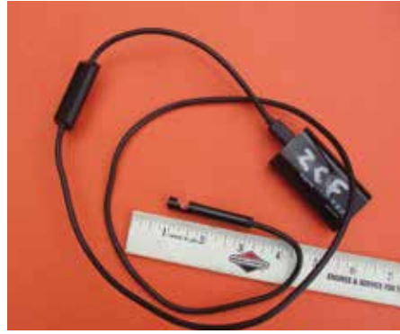
Above: This borescope fitted with periscope mirror connects to a wireless transmitter that shows up as the ZCF signal when mating with an Apple, Windows or Android phone, computer or other device.
