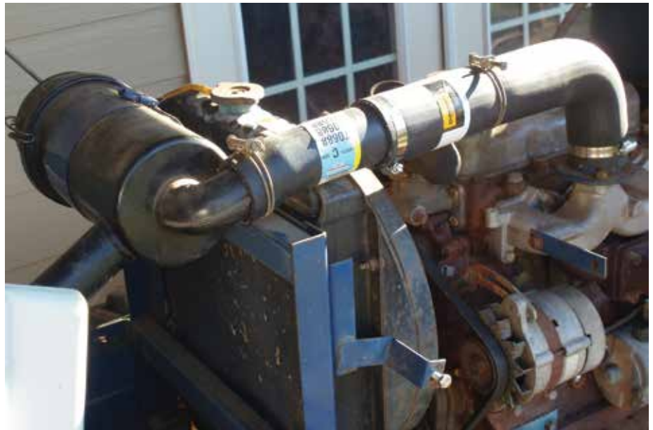
Two large-bore radiator hoses, with a steel pipe inside to reinforce the joint, formed a new intake air hose and put this 1978 Satoh tractor back in full operation.
