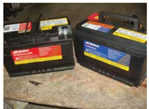
Of two batteries with equal power ratings, the AGM battery on the left is slightly smaller and lighter than the flooded-cell unit on the right.
