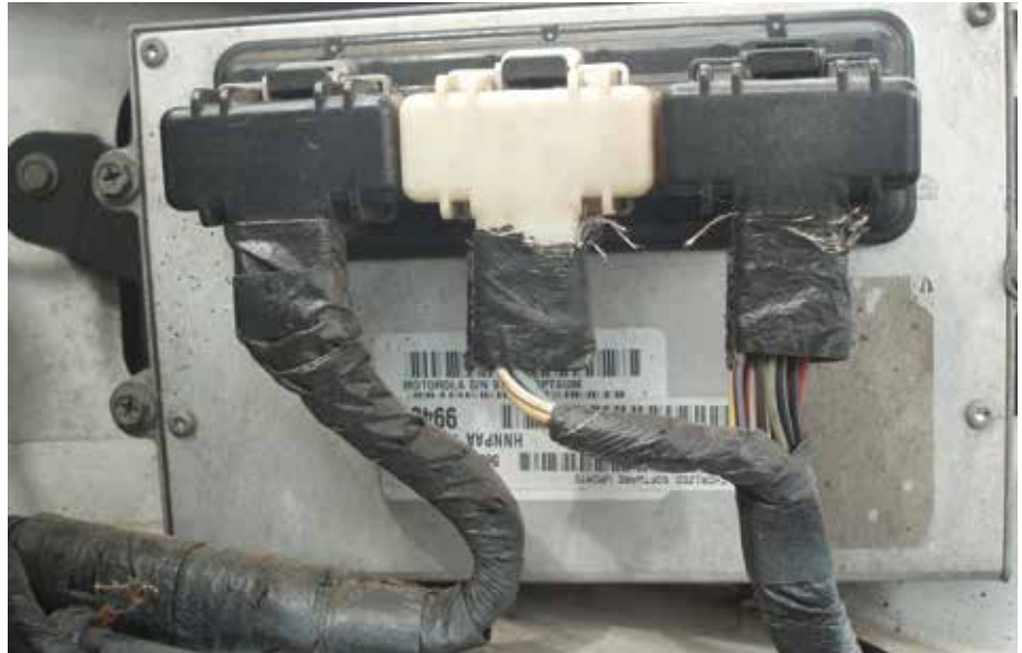
Engine control computer programs may reduce engine power and efficiency when a loose timing chain causes inaccurate data to come from input sensors. Photos by Scott R. Nesbitt
