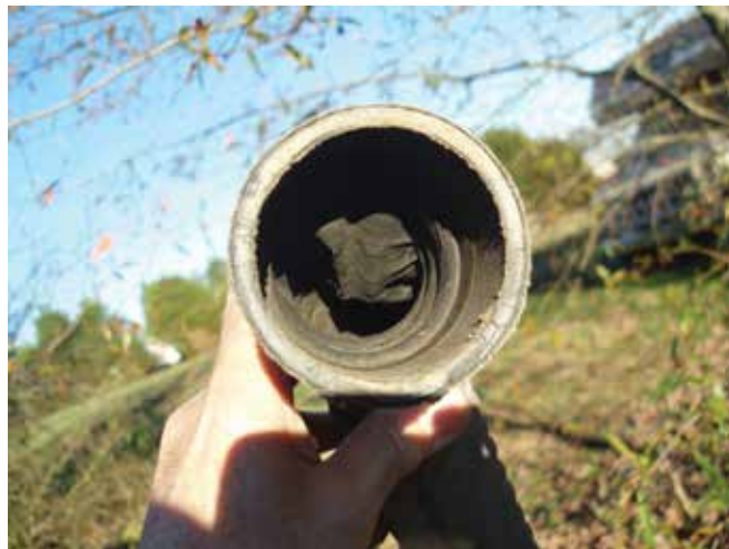
The inner liner of the air intake hose broke loose, partially blocking air to the engine and causing nasty clouds of black smoke and an inability to get above 1200 rpm. Photos by Scott R. Nesbitt
