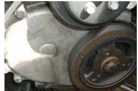
Replacing the timing chain set requires disassembling the front of the engine, and that may involve removing lots of chassis components.
