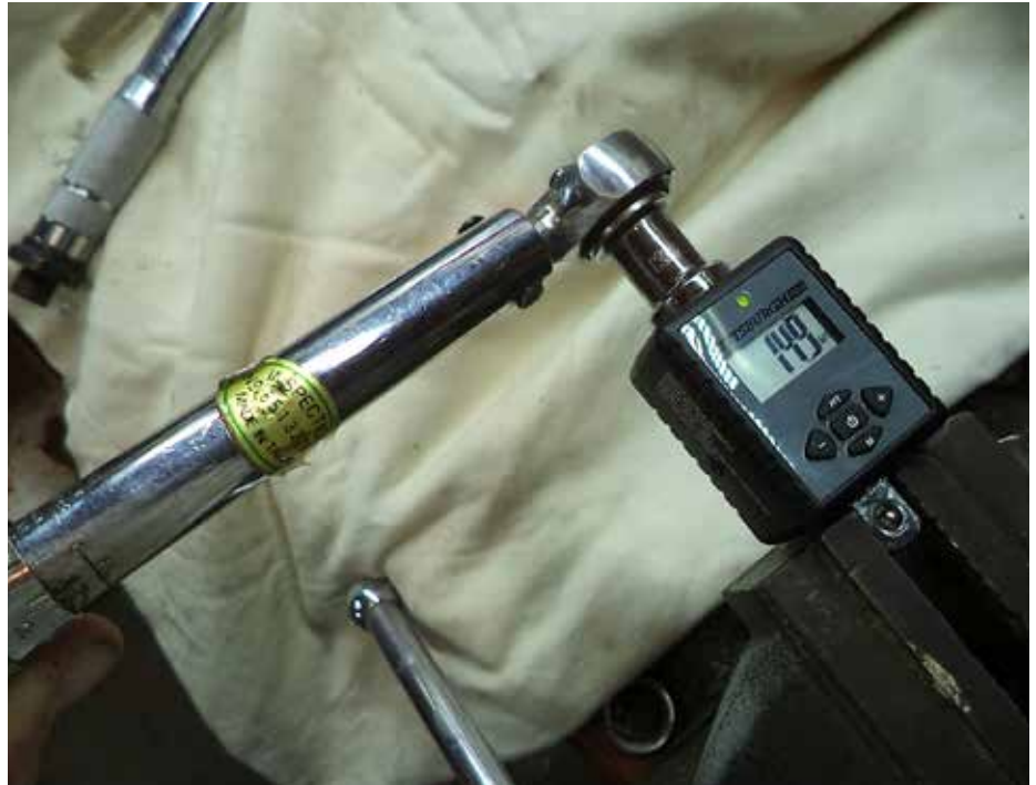
Clamping a digital torque adapter in a vise let us verify that the clicker-type torque wrench was clicking at 14.9 foot-pounds of torque when it was set for 15 foot-pounds. Such adapters can also be used directly to measure torque during machine assembly in the shop. Photo by Scott R. Nesbitt
