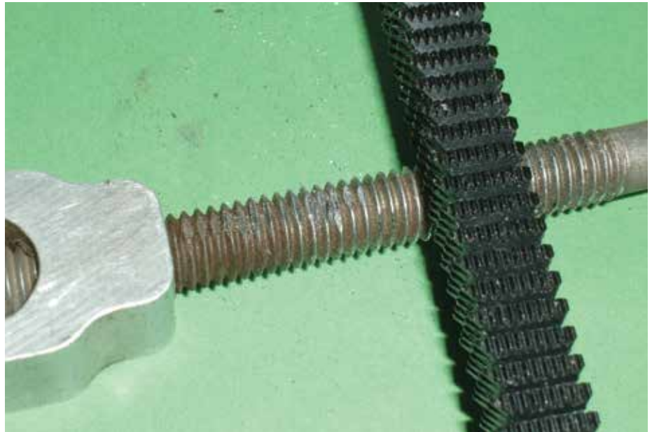
These threads were returned to usable condition in just a few seconds via a thread restoring file. Photos by Scott R. Nesbitt
