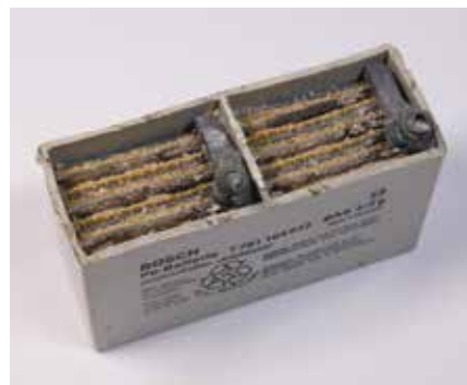
The gray and brown lead plates are separated and supported by the yellow and white glass fiber mats that are saturated with sulfuric acid in the two separate cells of this 4-volt AGM battery. Source: https://commons.wikimedia.org/wiki/File:Opened_AGM_battery.jpg
