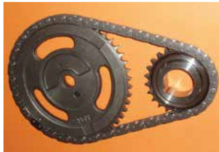
A chain-and-sprocket system coordinates crankshaft and camshaft positions to set the foundation for fuel, air and ignition control and adjustment.
