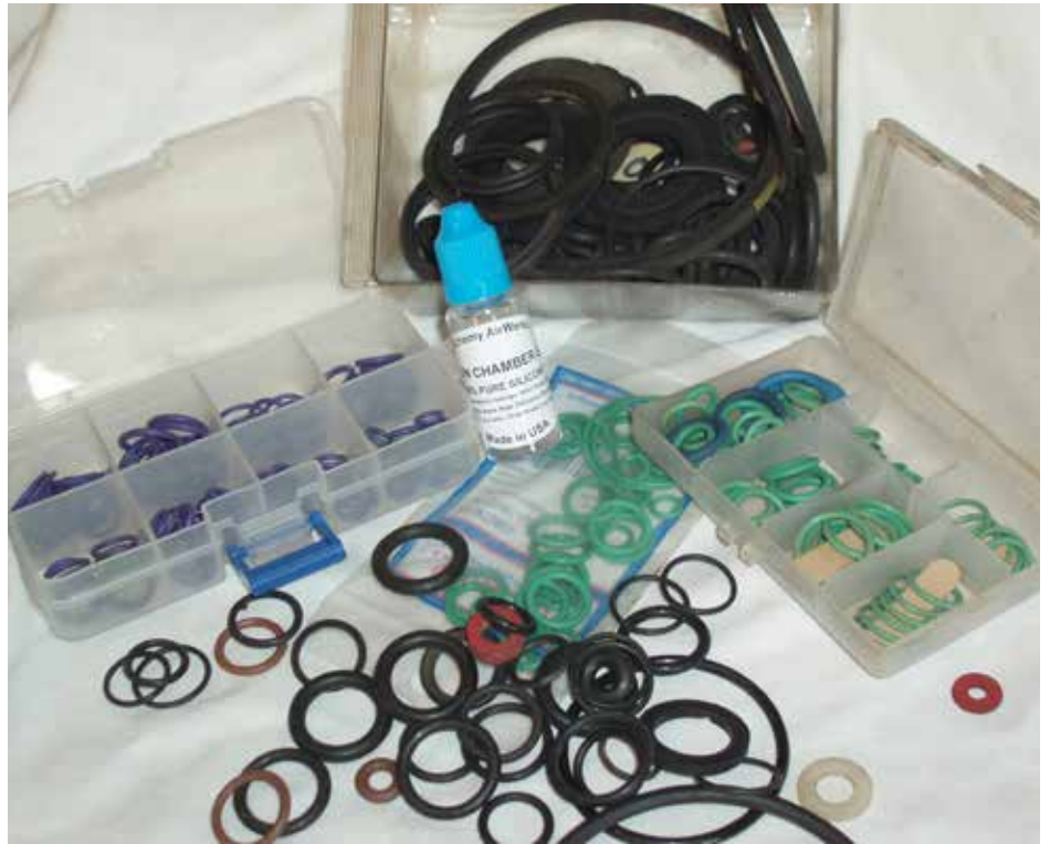
When searching for a "will fit" O-ring for a non-pressured, noncritical assembly like a hand-pump sprayer, the best choice is to look through the green and purple parts that are made of HNBR synthetic rubber and lubricated with pure silicone oil. There's no way to know what materials were used for the collection of O-rings that are left over from previous jobs. Photo by Scott R. Nesbitt
