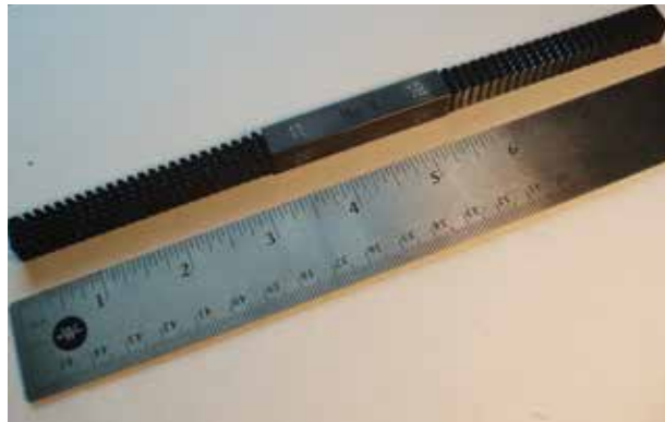
These threads were returned to usable condition in just a few seconds via a thread restoring file. Photos by Scott R. Nesbitt
